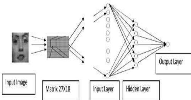
Fig . 2(a) . Architecture of proposed System
